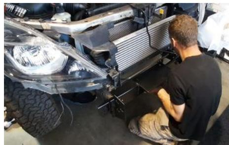
22. With help, mount the bar to the bracket with the supplied stainless steel hardware.
