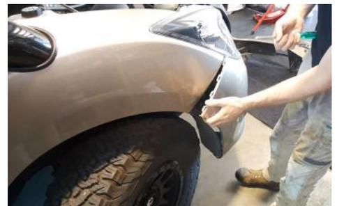
4. Remove the clips holding the top of the grill.
