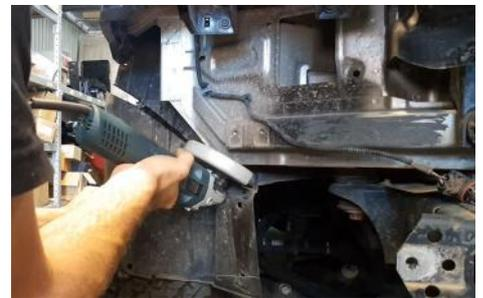
19. Remove the two piece plastic moulding below the headlights.
