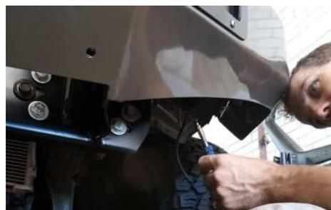
24. Using the two factory bolts for the rear and the supplied hardware for the front, mount your Extreme Series bash plate.
