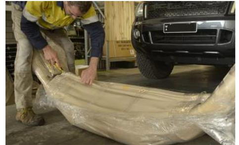
2. With the bar unwrapped, you're ready to remove the bumper. Start by removing the four clips either side holding the inner wheel lining to the bumper.
