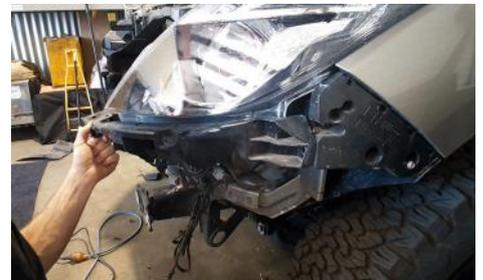
20. Strip the factory fog light wiring ready to solder on the new LED fog lights.
