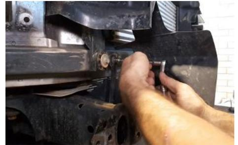
14. Tear away the plastic moulding that is between the chassis rail and the condenser.
