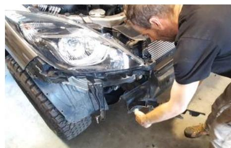
11. Unbolt the crash bar and dispose, this will be replaced by the bullbar mounts.
