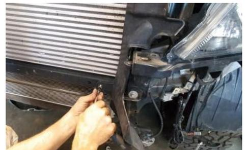
16. Trim the factory air dam as shown, cutting diagonally up.
