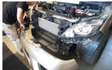
10. Tear away the plastic air dam on the impact bar.
