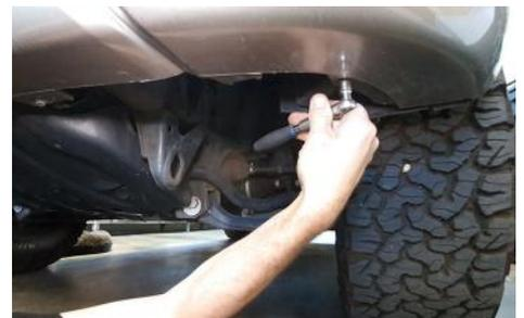
8. While you're down below, remove the factory bash plate, making sure you keep the two rear bolts to use later.
