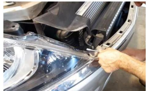
7. Undo the bolts holding the bottom of the bumper to the car.
