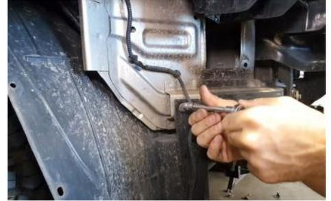
18. Trim the inner wheel liner as shown, following the angle of the metal.
